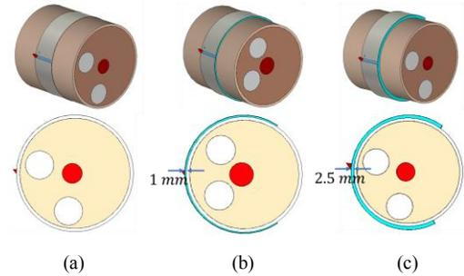
Fig. 2. Three scenarios of a GSM dipole antenna on a smart watch. (a) The dipole is placed underneath a dielectric watch strap and directly touches skin, (b) the dipole is placed on top of a dielectric watch strap, the strap thickness is 1mm, (c) the dipole is placed on top of a dielectric watch strap, the strap thickness is 2.5mm.
