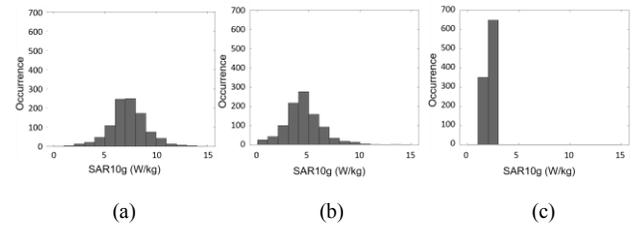
Fig. 3. Histograms of Monte-Carlo analysis with 1000 surrogate model evaluations in the cases of (a) the antenna underneath a strap, (b) antenna placed on top of a 1mm strap, (c) antenna placed on top of a 2.5mm strap.
