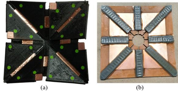
Fig. 3. Waterbomb antenna fabricated using: (a) copper tape and a flexible shell and (b) silicon encapsulated liquid metal hinges.
