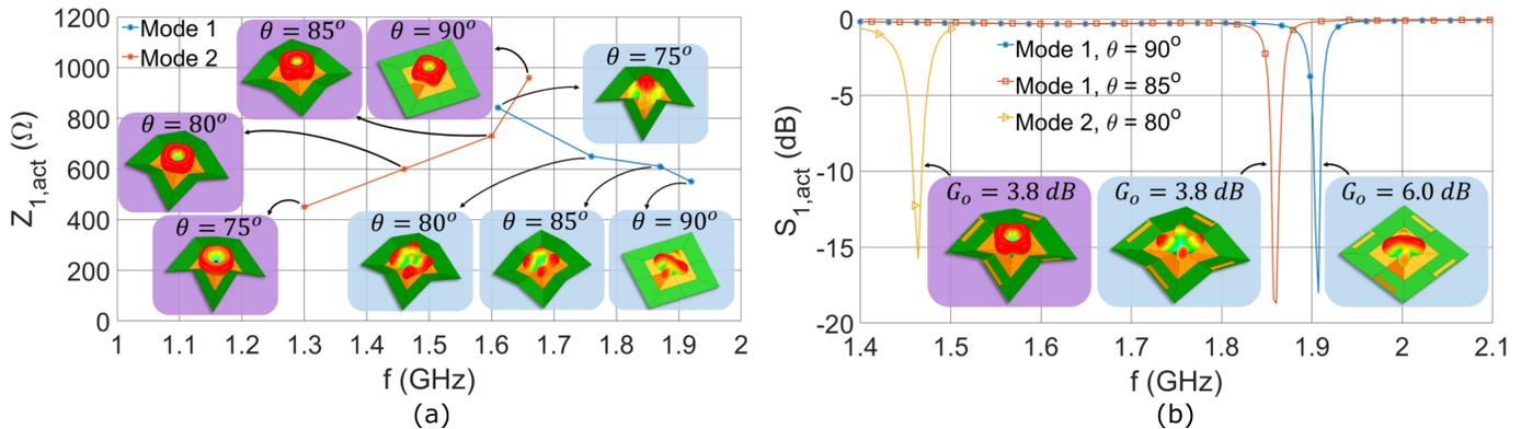
Fig. 2. (a) Simulated active input impedance, resonant frequency, and 3D radiation pattern of both modes as the antenna is folded/unfolded. (b) Simulated active scattering parameter of port 1 and 3D radiation pattern in three cases.
