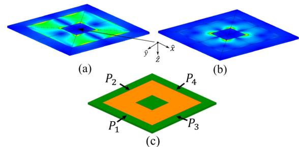
Fig. 1. Current distributions of: (a) mode 1, and (b) mode 2. Excitation locations are shown in (c).
