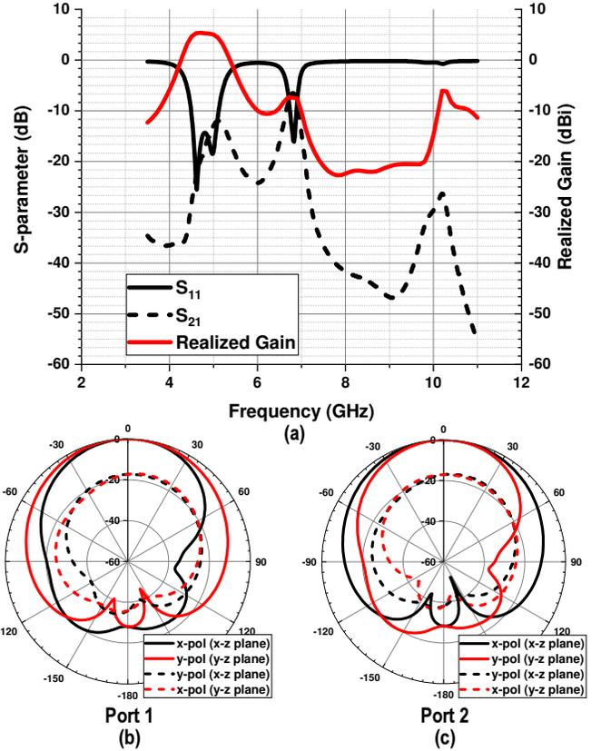
Fig. 3. (a) S-parameter and co-pol realized broadside gain responses. (b) The radiation patterns when fed at (b) Port 1 and (c) Port 2.
