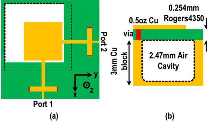
Fig. 2. (a) Dual-polarized FA top-view layout. (b) Metal/dielectric stackup cross-sectional view, where the single-layer PCB is placed on the Cu block, above the air-cavity carved within the Cu block denoted by the black dashed lines. The red rectangles represent vias to the Cu block.
