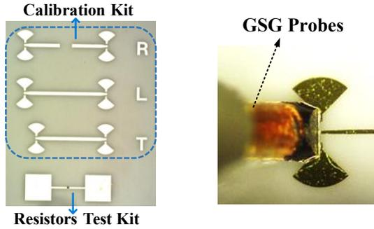
Fig. 2. A photo of the fabricated TRL calibration kit and the coplanar waveguide to microstrip line transition.
