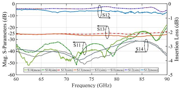
Fig. 4. The simulation and measurement results of S-parameters for the directional coupler with 25 dB coupling value.
