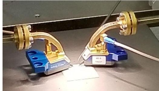
Fig. 1. A photo of a circuit under test using GSG coplanar probes.
