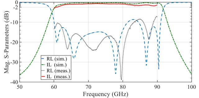
Fig. 6. The simulation and experimental results of S-parameters for the bandpass filter (RL: Return Loss, and IL: Insertion Loss).
