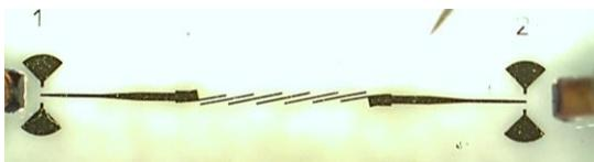
Fig. 5. A photograph of the fabricated E-band bandpass filter.
