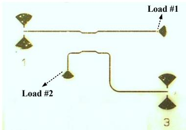
Fig. 3. A microphotograph sample of the fabricated directional coupler for measuring the coupling ( $S_{13}$ ) value.
