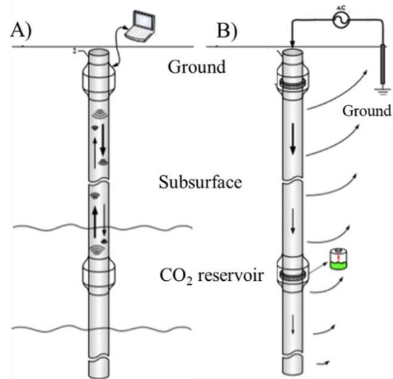
Fig. 1. (A) Schematics of wireless data transfer using toroidal antennas, and (B) wireless power transfer from surface to subsurface.
