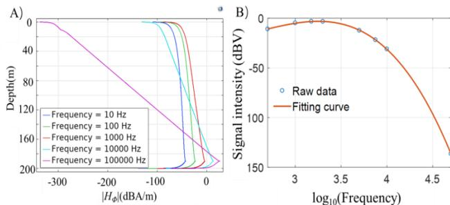
Fig. 2. Estimated  $H_\phi$  (A) and signal intensity (B) received on the surface w.r.t. working frequency
