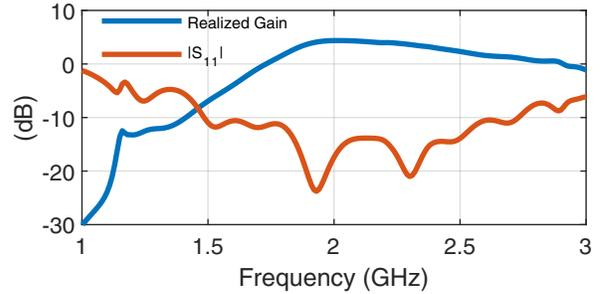
Fig. 4. Simulated realized gain and reflection coefficient.
