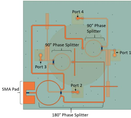
Fig. 2. Bottom view of the proposed antenna with semi-transparent substrates.
