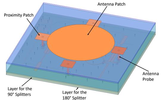
Fig. 1. Diagram of the proposed antenna with semi-transparent substrates.
