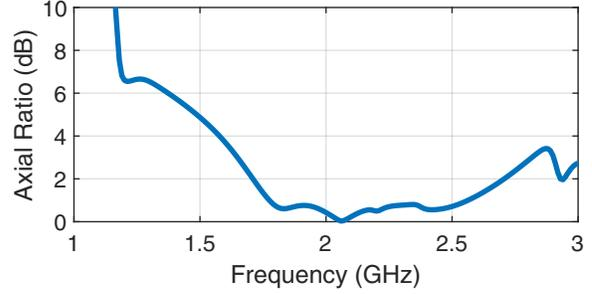
Fig. 3. Simulated axial ratio at broadside.
