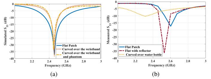
Fig. 3: (a) Simulated and (b) measured reflection coefficient of the proposed antenna for flat version and curved over wristband and human phantom.
