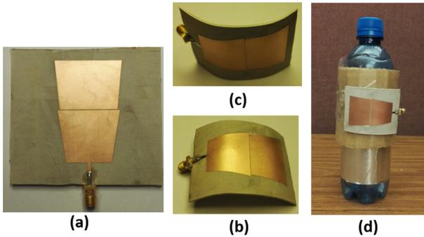
Fig. 2: Fabricated prototype of the proposed antenna. a)Top view b)Curved version top view. c)Curved version side view d) Setup used as the reflector and wristband.
