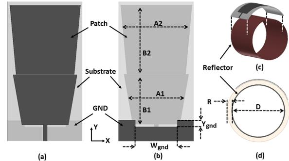
Fig. 1: Proposed curved antenna consisting two trapezoid patch and a reflector. a) Top view. b) Bottom view. c) Curved over a 60 mm diameter cylinder and 5mm away from the curved reflector. d) Side view.  $A1(\min - \max) = 21.8 - 29.7$ ,  $A2(\min - \max) = 27.5 - 32$ ,  $B1 = 25.2$ ,  $B2 = 23.5$ ,  $W_{gnd} = 20.2$ ,  $Y_{gnd} = 3.6$ ,  $R = 5$ ,  $D = 50$ , dimensions are in mm.
