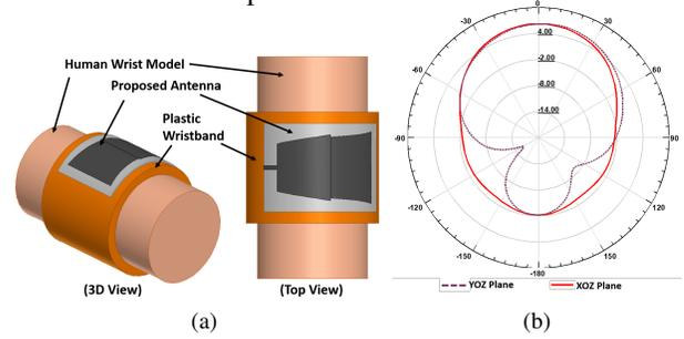
Fig. 4: (a) Simulated antenna over a plastic wristband and a body phantom and (b) Radiation gain of the proposed curved antenna in dBi.
