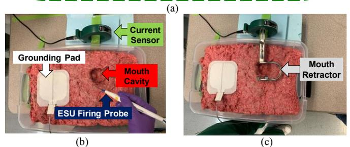
Fig. 1. (a) Schematic of experimental set-up which can be divided into two broad categories – Tonsillectomy and Sensing. Solid arrow lines depict physically connected entities or part of same entity, while dashed arrows depict no physical connection. (b) Experimental set-up without mouth retractor. (c) Experimental set-up with metal-based mouth retractor.
