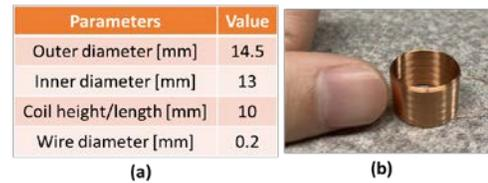
Fig. 1. (a) Relevant coil parameters. (b) Fabricated air-core coil sensor.
