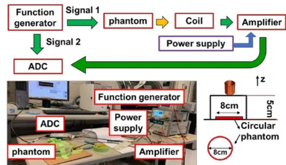
Fig. 2. Overall procedure and experimental set-up.
