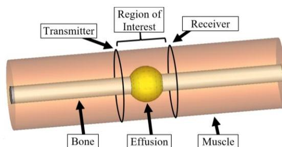
Fig. 1. Depiction of wearable conducting loops around arm model for detection and diagnosis of joint effusion size using change in electromagnetic propagation governing magnitude and phase of transmission between the loops.
