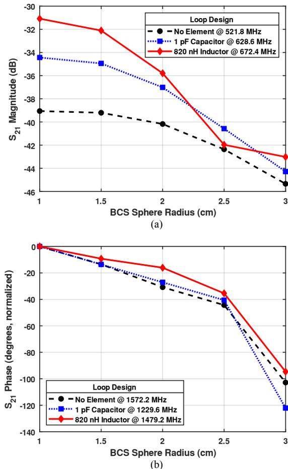
Fig. 2. Simulation results showing trends between  $S_{21}$  (a) magnitude or (b) phase and effusion radius. Each magnitude and phase plots consist of three cases, viz. no lumped element, lumped capacitor, and lumped inductor. The best result in magnitude is observed with a lumped inductor while the best result in phase is observed with no lumped element.
