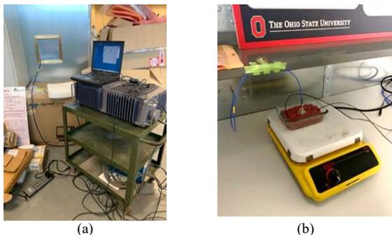
Fig. 1. Experimental setup: (a) wideband radiometer, and (b) hot plate used to heat the phantom.
