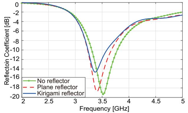
Fig. 2. Reflection coefficients of the antennas shown in Fig. 1 (a)-(c).
