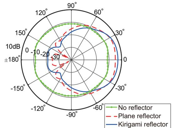
Fig. 3. Gain patterns in the  $x - y$  plane of the antennas shown in Fig. 1 (a)-(c).
