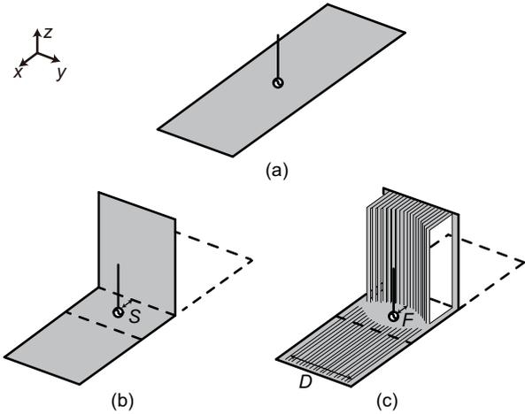
Fig. 1. The monopole antenna (a) without reflectors, (b) with one origami plane reflector, and (c) with one kirigami parabolic reflector ( $S = F = 21.4$  mm and  $D = 71.4$  mm).
