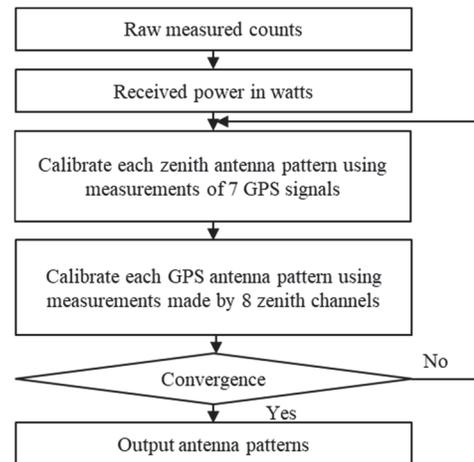
Fig. 1. Iterative antenna calibration approach.
