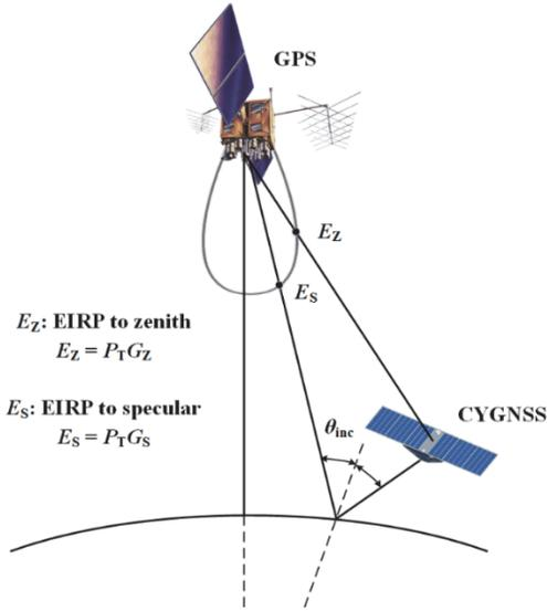
Fig. 2. Concept of the dynamic EIRP calibration algorithm.
