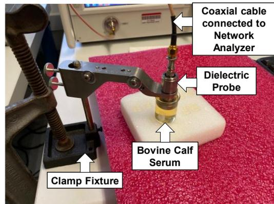
Fig. 1. Set-up for measurement of dielectric properties (permittivity and loss tangent) of bovine calf serum (BCS) sample using Keysight's high temperature probe N1501A-101 and a network analyzer.
