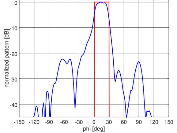
Fig. 3. Pattern from (blue) proposed method and (red) sector beam specification.  $\theta = \pi/2$  plane.
