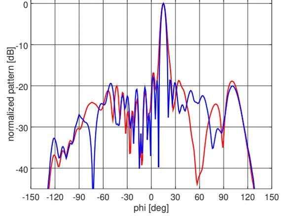
Fig. 2. Pattern from (blue) the proposed method for the “impulse beam” specification and (red) unconstrained “phase-only” beamforming.  $\theta = \pi/2$  plane.
