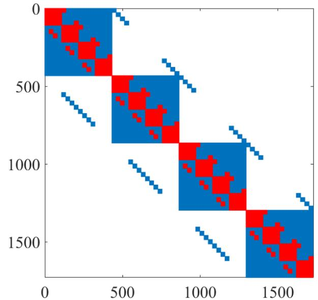
Fig. 1. Sparsity pattern of the stiffness matrices in a  $4 \times 4 \times 4$  domain. The global stiffness is in blue; the sub-domain matrices are in red.
