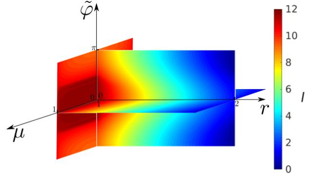
Fig. 2. Contour plot of radiation intensity of the benchmark problem for  $R_1/R_2 = 0.5$  and  $\tau_2 - \tau_1 = 10$ .
