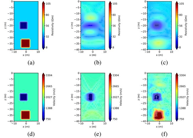
Fig. 2. Demonstration of the joint inversion results. (a) and (d) are the true models. (b) and (e) are the separately inverted models, (c) and (f) are the jointly inverted models.
