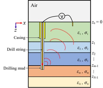
Fig. 1. Schematic of EM telemetry system in layered media.
