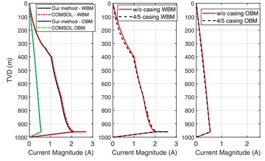
Fig. 2. Magnitude of electric current distribution on a 1000 m vertical drill string. Left subplot: current distribution for two cases: WBM–casing coating; OBM–casing coating; Central subplot: casing length effect for WBM–casing coating; Right subplot: casing length effect for OBM–casing coating.
