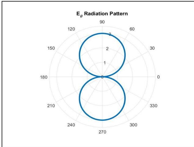
Fig. 2. Radiation pattern of a folded unipole antenna with a single fold and a tower.
