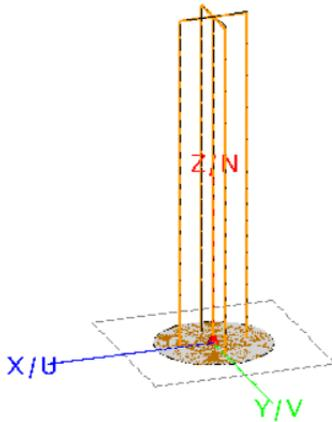
Fig. 3. Preliminary model with 4 cables using CADFEKO
