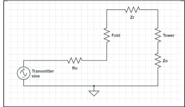
Fig. 1. Equivalent circuit of a folded unipole antenna.
