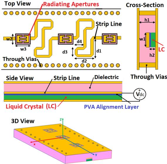
Fig. 1. Schematic of the LC based LWA.
