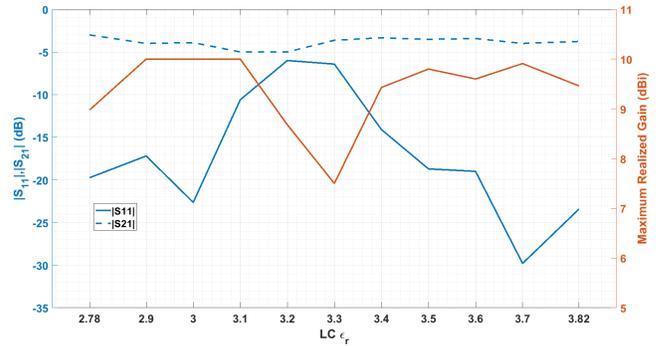
Fig. 3. S parameters and maximum realized gain at each scan (LC relative permittivity) for the proposed LC-based LWA.
