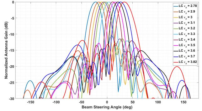
Fig. 2. The beam scanning angle of  $56^\circ$  with side lobes less than -10 dB is obtained.
