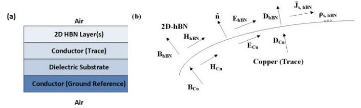
Fig. 1. (a) Cross section of a 2-D hBN coated microstrip RF circuit, (b) Fields at a general interface between 2-D hBN and Copper.
