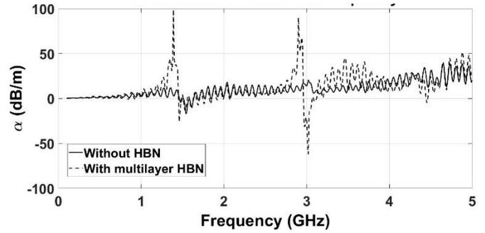
Fig. 5. Comparison of attenuation constant in dB/m vs. frequency in GHz for prototyped transmission lines.
