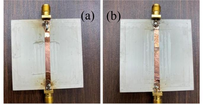
Fig. 2. 50  $\Omega$  Transmission Line with (a) 2-D hBN coated copper and (b) blank copper on the Rogers TMM4 substrate.
