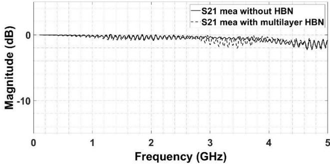
Fig. 4. Comparison of the magnitude of transmission coefficient in dB vs. frequency in GHz for prototyped transmission lines.
