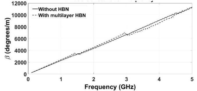
Fig. 6. Comparison of phase constant in degrees/m vs. frequency in GHz for prototyped transmission lines.
