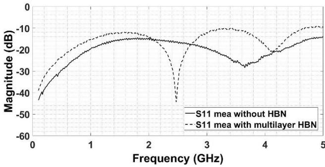
Fig. 3. Comparison of the magnitude of reflection coefficient in dB vs. frequency in GHz for prototyped transmission lines.
