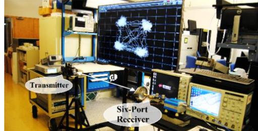
Fig. 5. The V-band wireless link experimental setup.
