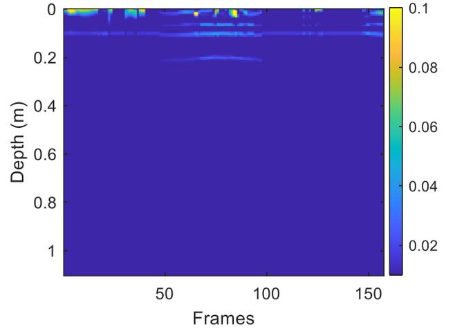
Fig. 2. B-Scan of a metal plate under concrete slabs after applying elliptical-windowing clutter-pole removal.
