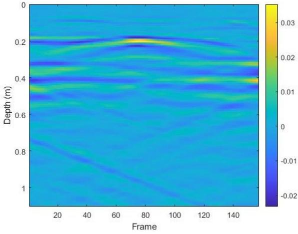
Fig. 1. B-Scan of a metal sheet under concrete slabs using background removal.
