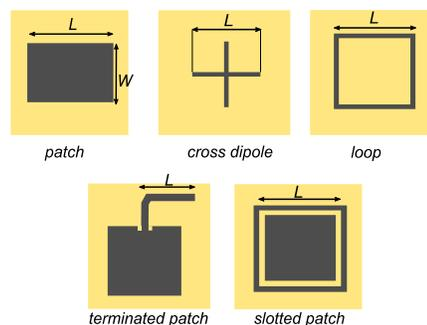
**Figure 1** Typical RA unit cell geometries.
