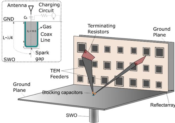
**Figure 2** Sketch of the assembly SWO+RA.
