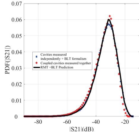
Figure 4: BLT formalism results for three cascaded interconnected cavities.
