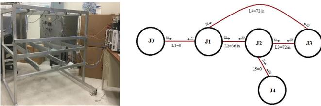
Figure 3: Left: Experimental set-up for three networked cavities; right: BLT topological network for three randomly interconnected cavities.
