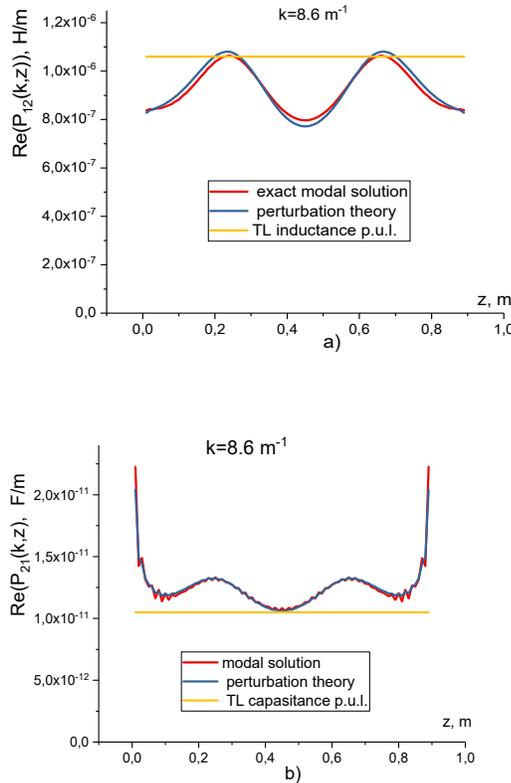
Fig. 2. Length dependence of the  $P_{12}$  (inductance-like) and  $P_{21}$  (capacitance-like) elements of the parameter matrix for the high-frequency case far from the cavity resonances.  $k=8.6\text{m}^{-1}$ .
