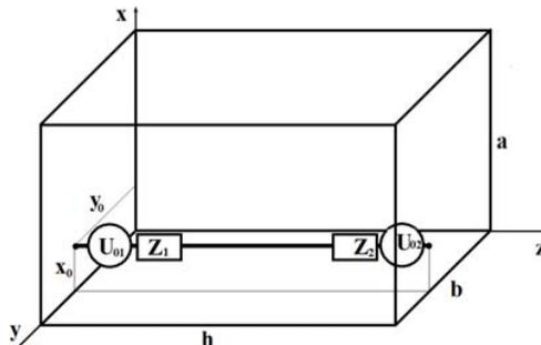
Fig. 1. Loaded thin-wire line with symmetrical geometry in a rectangular resonator (Resonator:  $a=1.5\text{m}$ ,  $b=1.2\text{m}$ ,  $h=0.9\text{m}$ ; Transmission line:  $x_0=9\text{cm}$ ,  $y_0=37\text{cm}$ ,  $r_0=1\text{mm}$ ).
