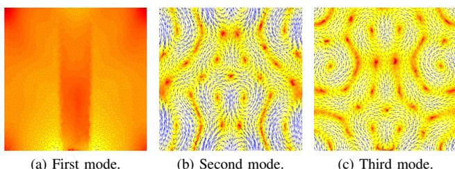
Fig. 2. Spatial distributions of the first three electric field modes. The first mode is a simple straight beam mode reminiscent of when the injected current is below the space charge limit, while the second and third modes display cavity configurations induced by the coherent oscillation of the electrons.
