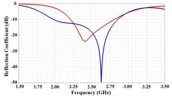
Fig. 4. Reflection coefficient of the primary (blue curve) and one of the secondary (red curve) antennas.
