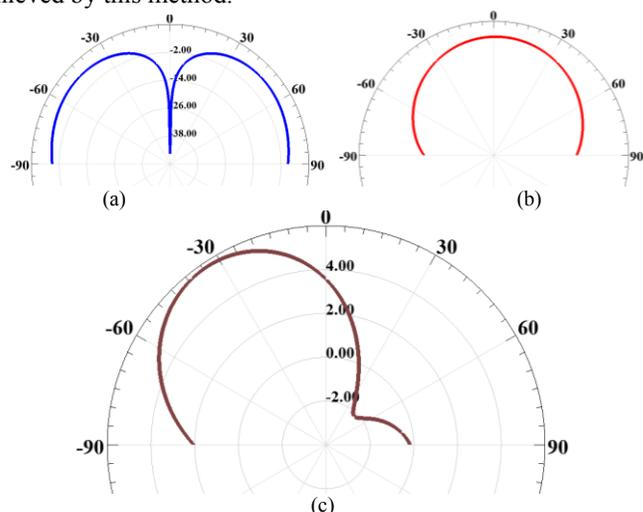
Fig. 2. (a) The radiation pattern of the DR at the  $HEM_{11\delta}$  mode, (b) radiation pattern of a secondary excitation by using a monopole antenna, and (c) super composition of the two excitations.
