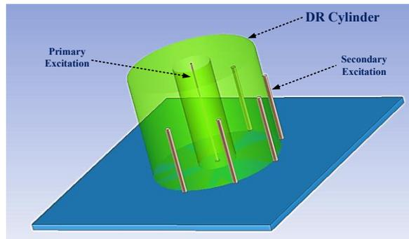
Fig. 1. Configuration of the proposed beam steering antenna by dielectric resonator antenna
