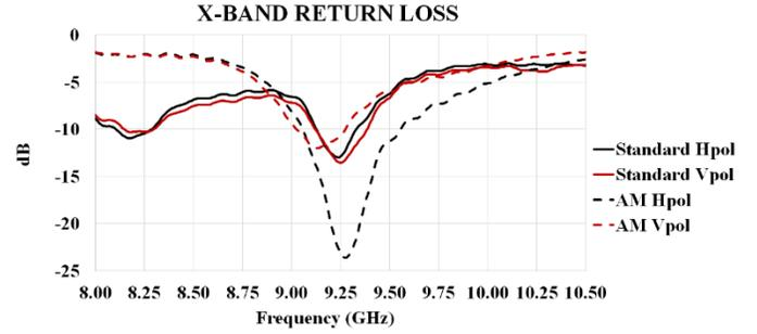
Fig. 4. Comparison of X-band return loss for the antennas shown in Fig. 2a and Fig. 2b.
