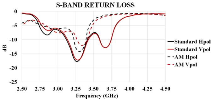
Fig. 3. Comparison of S-band return loss for the antennas shown in Fig. 2 and Fig. 2b.
