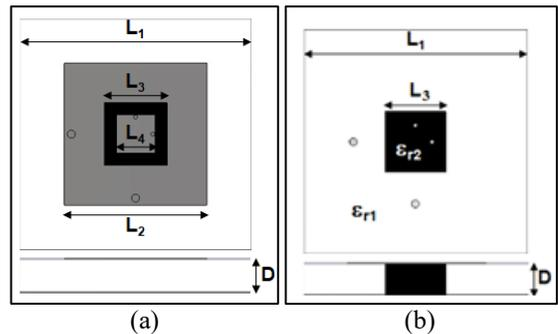
Fig. 1. a) Layout of the dimensions of the S/X-band antenna and b) layout of the hybrid dielectric substrates.
