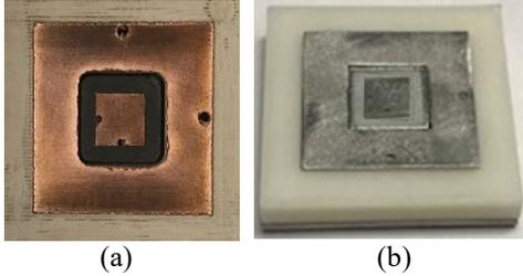
Fig. 2. a) Top view of the traditional copper plated antenna and b) top view of the AM version of the same antenna.
