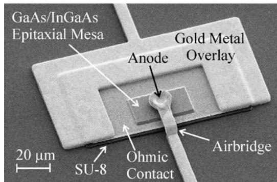
Fig. 1. Scanning electron micrograph of a heterogeneously-integrated quasi-vertical Schottky diode.
