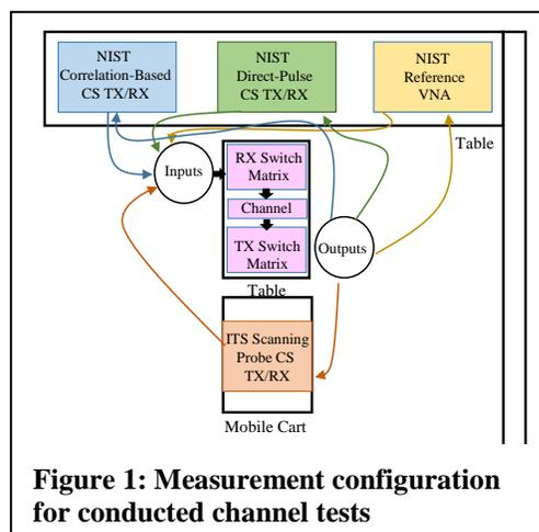
**Figure 1: Measurement configuration for conducted channel tests**
