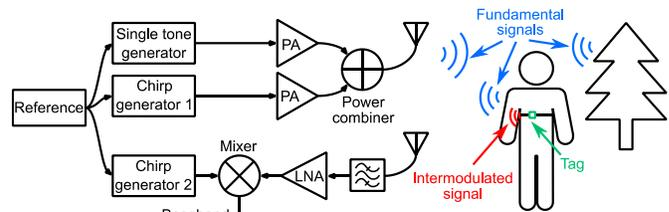
Fig. 1. Top level block diagram of the IM-FMCW radar.
