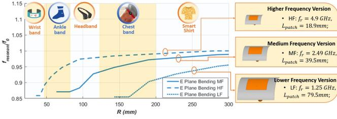
Fig. 3. Normalized frequency shift ( $f_{res}/f_0$ ) with respect to bending radius  $R$ , targeting at various potential wearable applications.
