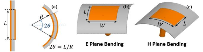
Fig. 1. Characterization of rectangular patch antenna bending effects. (a) The illustration of bending angle  $2\theta$  and bending radius  $R$ . The E plane bending and H plane bending cases are shown in (b) and (c), respectively. The patch dimensions  $L$  and  $W$  are kept constant as  $2\theta$  and  $R$  are varied throughout the study.
