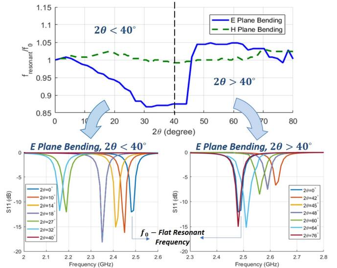
Fig. 2. Frequency variations of the bending effects on both E and H plane. The normalized frequency shift is plotted with respect to bending angles for the rectangular patch antennas. The E plane frequency shift due to bending splits into two regions, with left shift on slightly bent region ( $2\theta < 40^\circ$ ), and right shift on severely bent region ( $2\theta > 40^\circ$ ).
