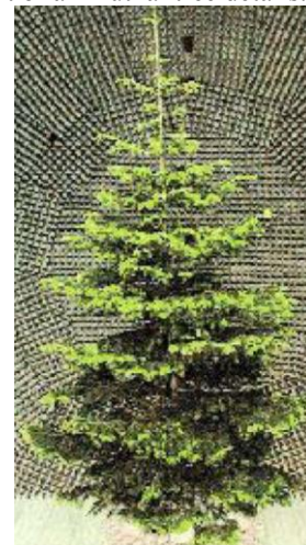
Figure 1. Caucasian FIR tree ( Abies Normanniana ) in an anechoic chamber at the EMSL JRC in Ispra, Italy [11].
