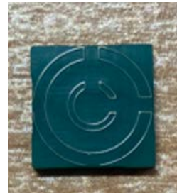
Figure 2: Prototype of the unit cell featuring concentric circular split-ring resonators (C-SRR).
