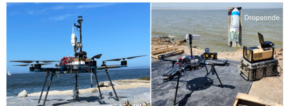
Fig. 2. OSU Drone Receiver systems where the left side shows the Hexacopter and right side shows the tethered Quadcopter setup.
