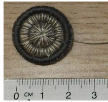
Figure 2. The E-textile electrodes suitable for wearable devices and knitted on the desired objects.
