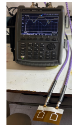
Figure 6. Measuring the scattering parameters with Agilent Technologies Microwave Analyzer, N9916
