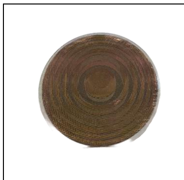
Figure 1. Fabricated quad-beam lens antenna.
