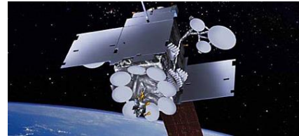
Fig. 1. The Inmarsat 5F4 satellite antenna farm (artist impression)
