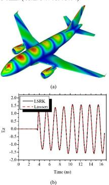
Fig. 1. Scattering of a plane wave by an aircraft at 600MHz obtained by the DGTD- $\mathbb{P}_2$  method based on the combined Lawson-LSRK scheme: (a) a top view about the contour lines of the Fourier transform of the electric field. (b) time evolution of  $E_*$  of a given point obtained.
