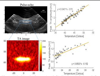
Figure 1. Pulse-echo image (top left), TA image (bottom left) from matching layer-saline interface and change in peak TA signal with temperature for saline (top right, r=0.948) and porcine tissue sample (bottom right, r=0.876). Data points (o) and fitted line (solid line).
