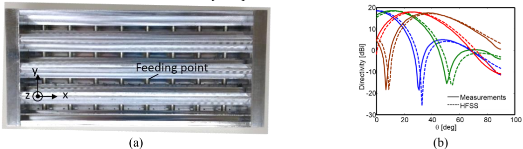
Figure 1. 8×4 Array of long slots. (a) Front view of the prototype. The coaxial-probe transition is labeled as a feeding point. (b) Directivity in the xz-plane for scanning at \theta=0^\circ , 15^\circ , 30^\circ and 45^\circ at 5.8 GHz. Simulation results from Ansys HFSS are shown for comparison.
