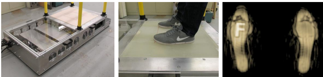
Figure 1. (left) PNNL mm-wave shoe scanner laboratory prototype system, (center) scan of mock passenger wearing sneakers, (right) example mm-wave imagery revealing F-target located inside shoe.
