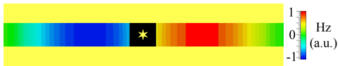
Fig. 2. The magnetic field distribution inside of the plasmonic cloak for the TM incidence.
