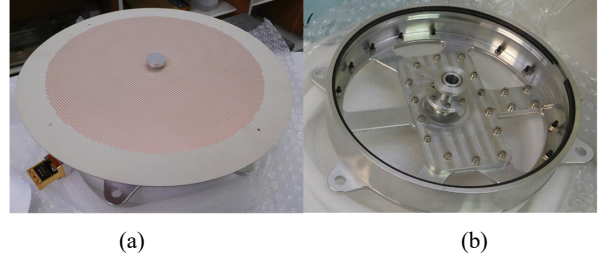
Fig. 3: Realized prototype. (a) Radiative panel mounted on the feeding structure (bottom-left corner: the input RW). (b) Rotating feeding structure (at the center: CW exciting the SW on the radiative panel).
