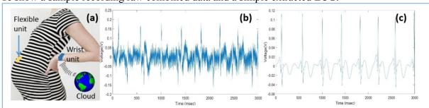
**Figure 1. a)** Conceptual design of the system. **b)** Raw data of a recorded combined ECG mimicking that of f/mECG and **c)** A de-noised and extracted ECG using the other ECG as the reference signal.
