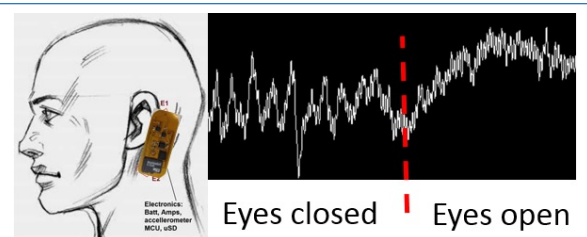
Figure 1. Conceptual design of the EEG patch and a regular eyes closed-open recording showing PDR.
