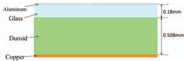
Fig. 1. Cross sectional view of coplanar waveguide on microstrip line.
