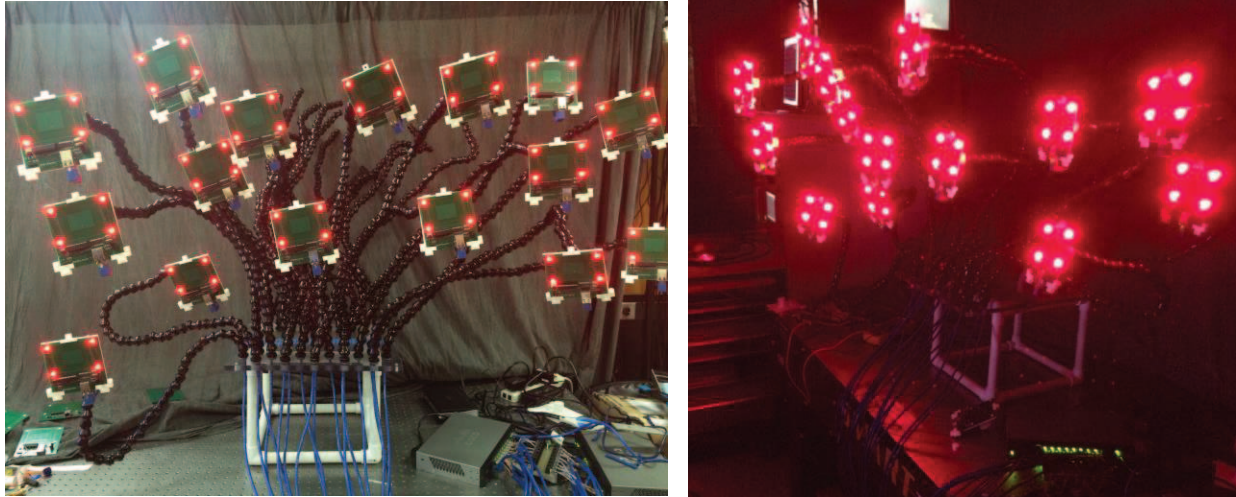
Figure 15. (Left) 16 element random array test apparatus (Right) Side view of test apparatus
